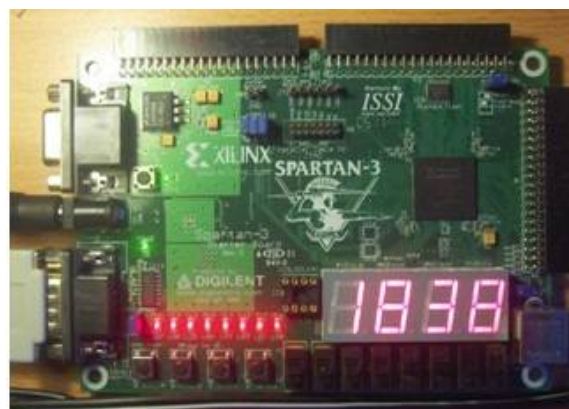
Fig9: Spartan FPGA board
